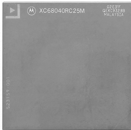
Photo of a Motorola 68040 processor taken by Konstantin Lanzet. Shared under CC BY-SA 3.0 license at https://en.wikipedia.org/wiki/Motorola_68040 .
